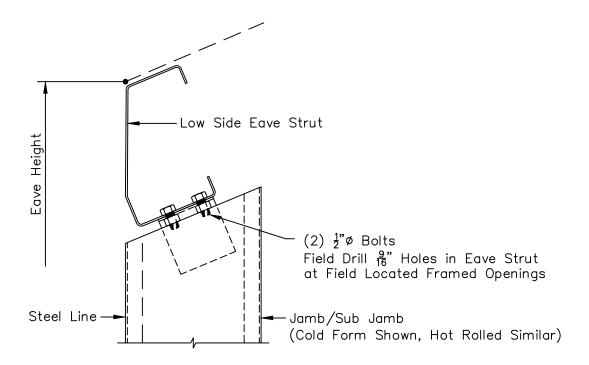
Jamb/Sub Jamb to Low Side Eave Strut 49:12 thru 12:12 Roof Slope
